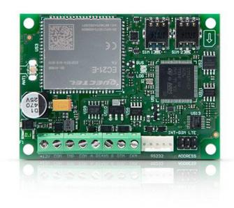
A big advantage of INT–GSM LTE device is the ability to work with the **ETHM–1 Plus** Ethernet module (RS–485 port connection). The duo allows for realization of Dual Path Reporting, in accordance with EN 50136, as well as for determining the priority of event monitoring tracks (Ethernet, cellular data and SMS). By default, cellular network is a backup communication channel for Ethernet.
